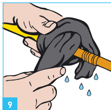
9 Wrap exposed plastic with a damp cloth
