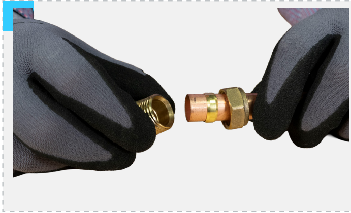
1. Remove the nut and olive from the fitting.
